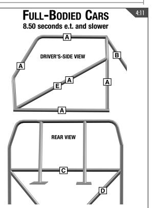
All cars with an OEM frame must have roll cage welded to frame.
