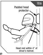
alone is not acceptable as a padded head protector unless it is within 4 inches of the driver's helmet. A seat that incorporates a reinforced head rest is permitted.
